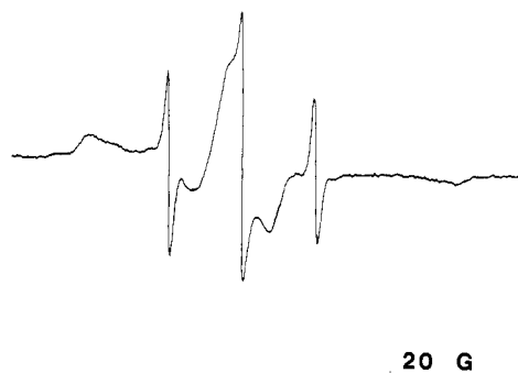
Figure 3. Spectrum of the PEO 1000 grafted on silica with a low grafting ratio ( S = 0.17 molecule/nm 2 or S = 0.04 molecule/ \text{\AA}^2 ) at 22 °C in C 6 H 6 .
